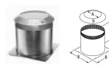
Use in installations that pass through an attic to prevent insulation and debris from accumulating near the chimney, unless chimney is enclosed through attic. Fits over Firestop Radiation Shield or a support box. Consists of two parts – a collar and a base. Mesh sleeve around top.
