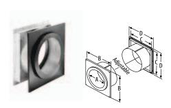
Use to provide clearance to combustibles. Adjusts from a minimum of 4" to a maximum of 10" wall thickness, and fits between standard wall studs. To accommodate thicker walls, the telescoping pieces can be extended up to 16" with a fieldfabricated extension installed. Interior trim ring painted black. Must be installed with DuraTech chimney pipe horizontally through the wall and extend 6" into the room beyond the interior wall.
