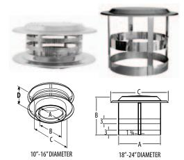
Required where pipe terminates above the roof line. Removable screws allow for cleaning of the chimney and spark arrestor screen. Made of stainless steel.
