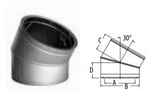
Use for offsets around obstructions such as rafters, ridgepoles, or joists. May have one pairs of elbows if needed. Offsets greater than 30° are not permitted in accordance to UL 103 standards. Large diameters are restricted to one pair of elbows.
