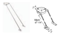
Use to support the chimney when it extends more than 5' above the roof. Provides stability to chimney against wind and snow. Mounting brackets and adjustable tubing included.
