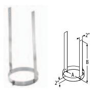
Use to prevent excessive weight on the elbows by supporting the weight of the chimney. Required to be installed between two elbows in offset installations. Multiple elbow straps may be required for offset installations. Refer to installation instructions.
