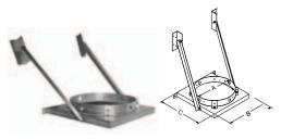
Use as wall support for chimney system. Supports up to 30' of DuraTech Chimney. Attaches to chimney pipe. Can be installed above or below the Tee. If installed below the Tee, a short section of pipe is required.
