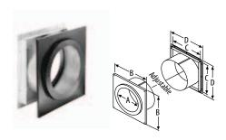
Adjusts from a minimum of 4" to a maximum of 10" wall thickness, and fits between standard wall studs. To accommodate thicker walls, the telescoping pieces can be extended up to 16" with a field-fabricated extension installed. Interior trim ring painted black. Must be installed with DuraTech chimney pipe horizontally through the wall and extend 6" into the room beyond the interior wall. (Black painted DuraTech is available). 6" and 8" stainless steel exterior trim available.
