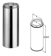
5" - 8" Diameters - Designed for appliances that are tested and listed for use with a 2100° F HT chimney system, such as wood stoves, fireplaces, furnaces, boilers, ranges, water heaters, or other appliances fueled by wood, oil, coal, or gas. Tested to UL test procedures 103 HT and listed under UL re-examination service number MH 7399. Available in stainless steel (SS) or in a galvalume (GA) outer casing and stainless steel inner wall with twist-lock connections.
