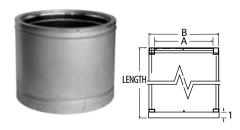
To calculate installed length of 10", 12", 14", 16", 18", 20", 22" or 24" DuraTech Chimney, subtract 3/4" from each joint overlap of chimney pipe. Important: Allow a minimum of 2" air space to combustibles when installing DuraTech Chimney.
