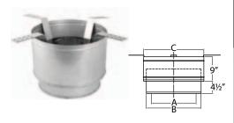
Supports chimney pipe and provides a positive connection between support box and chimney with a built-in twist-lock. Supports up to 40' of DuraTech Chimney. Trim collars are sold separately. (For 10" use DuraBlack Slip Connector to attach DuraBlack to the support box. See DVL/DuraBlack section).
