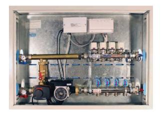
The ThermalPro Isotherm Mixing Module is a compact, pre-piped, pre-wired pump and mixing valve control connected directly to a Watts Radiant 1" Standard or 1-1/2 Hi-Flow Stainless Steel manifold and installed in a white powder coated steel cabinet with cover door.
