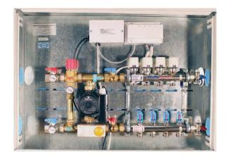
The ThermalPro Isotherm Mixing Module is a compact, pre-piped, pre-wired pump and mixing valve control connected directly to a Watts Radiant 1" Stainless Steel manifold and installed in a beautiful white powder coated steel cabinet with cover door.
