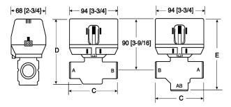
Fig. 1. Nominal dimensions in inches [millimeters]
