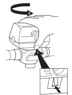
Fig. 7. Lock Mechanism to detach Actuator
