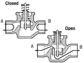
Fig. 2. Fluid Flow of 2-way valves
