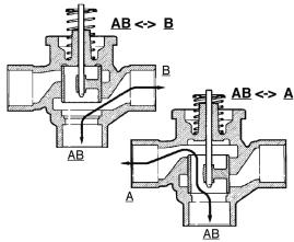
Fig. 3. Fluid flow of 3-way valves
