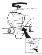
Figure 7 - Lock Mechanism to detach Actuator
