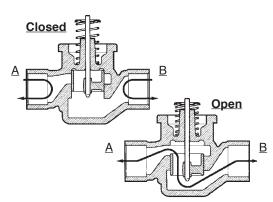
Figure 2 - Fluid flow of 2-way valves
