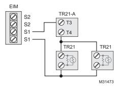
Fig. 358. Wiring 2 TR21 sensors and 1 TR21-A sensor.
