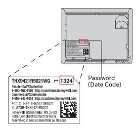
Fig. 54. Finding thermostat password.
