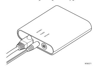
Fig. 47. RedLINK Internet Gateway connect button.
