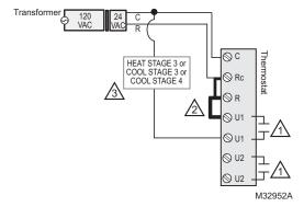
Fig. 331. Prestige THX9321 powering universal relay with system transformer.
