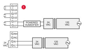
Fig. 344. Wiring a powered humidifier.
