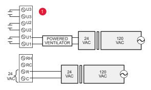
Fig. 345. Wiring a powered ventilator.
