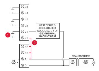
Fig. 350. Connecting a stage of heating or cooling to a universal relay (U1, U2, U3).
