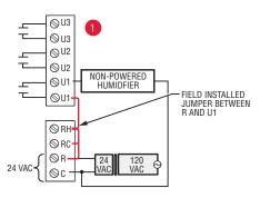
Fig. 347. Wiring a non-powered humidifier.
