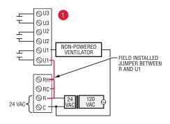
Fig. 348. Wiring a non-powered ventilator.
