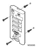
Fig. 73. Mounting Entry/Exit Remote or Vent Boost Remote.
