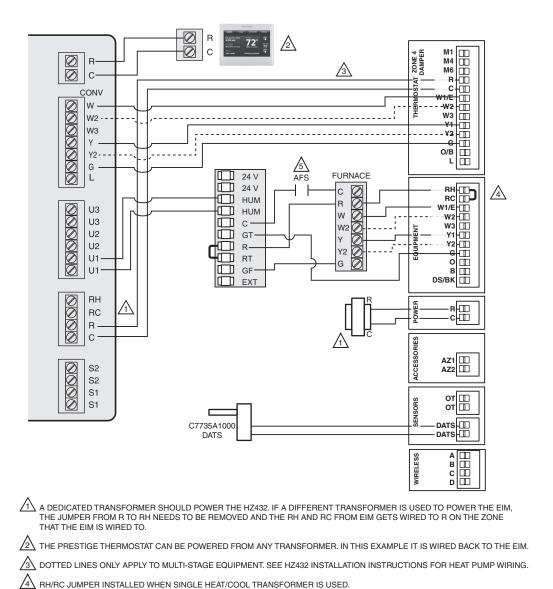
Fig. 362. Prestige IAQ controlling one zone with an HZ432 zone panel and a TrueSTEAM humidifier.
