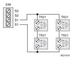
Fig. 359. Wiring 4 TR21 sensors.
