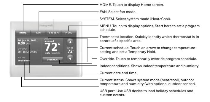
Fig. 75. Quick reference to commercial display.
