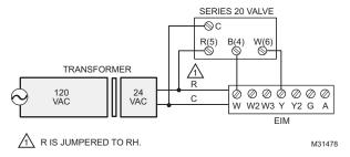
Fig. 334. Series 20 hot water heat.
