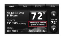
Fig. 313. Reading temperature at the Portable Comfort Control.
