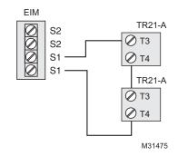
Fig. 360. Wiring 2 TR21-A sensors.
