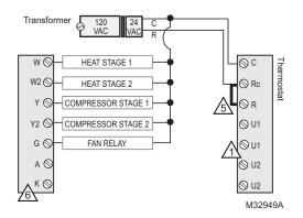
Fig. 328. Prestige THX9321 and 2-heat / 2-cool conventional system with one transformer.
