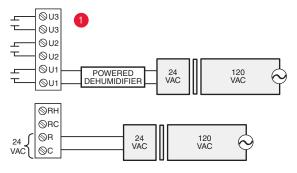
Fig. 346. Wiring a powered dehumidifier (whole house dehumidifer).
