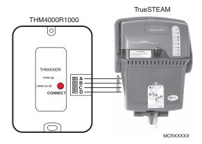
Fig. 48. Connect button on TrueSTEAM wireless adapter.
