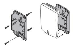
Fig. 70. Mounting Indoor Sensor.
