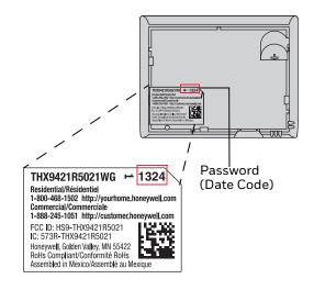
Fig. 6. Finding thermostat password.
