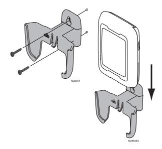
Fig. 68. Mounting Outdoor Sensor.
