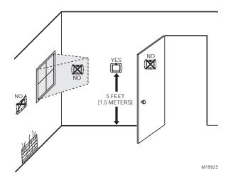
Fig. 16. Selecting thermostat location.
