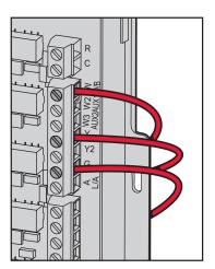
Fig. 323. Inserting wires in EIM terminal block IMPORTANT
