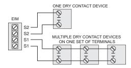
Fig. 187. Wiring dry contact devices.
