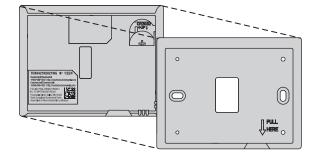
Fig. 17. Separate wallplate from thermostat (THX9421).
