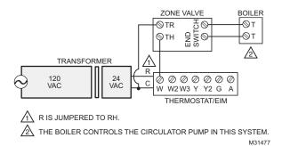
Fig. 333. 2-Wire Zone Valve with end switch.
