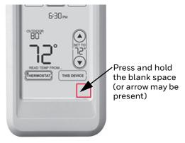
Fig. 46. Restarting the linking process.
