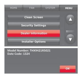
Fig. 55. Finding thermostat password.
