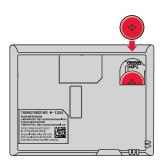
Fig. 19. Insert coin cell battery (THX9421)
