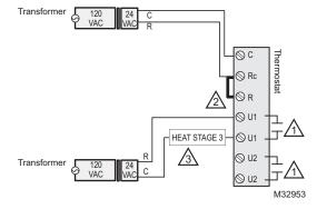
Fig. 332. Prestige THX9321 powering universal relay with separate heating transformer.
