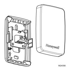
Fig. 71. Remove the cover.
