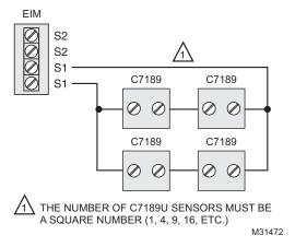
Fig. 357. Wiring 4 C7189U sensors.
