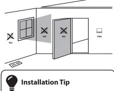
Pick an installation location that is easy for the user to access. The temperature of the location should be representative of the building.
