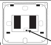
Gas: For systems that control the fan during a call for heat, put the fan operation switch to the GAS position. **Electric**: For systems that do not control the fan during a call for heat, put the fan operation switch tothe ELECTRIC position.
