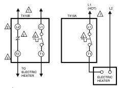
POWER SUPPLY. PROVIDE DISCONNECT MEANS AND OVERLOAD PROTECTION AS REQUIRED.
