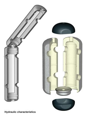
The hydraulic separator should be sized according to the maximum flow rate value at the inlet. The selected design value must be the greatest required flow rate of either the primary circuit or the secondary circuit.
