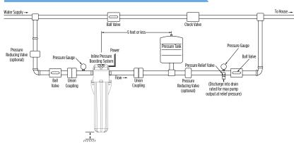
\*It is recommended (where applicable) to install the Inline 400 in PARALLEL with the incoming water supply. This will allow for a "service bypass" so that the typical household can still utilize the incoming water (although at a reduced pressure) if maintenance work is required. This type of installation requires a ball valve be installed as shown above.
