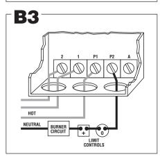
**B3** Connect terminal P2 to burner circuit in series with and before other limit controls.
