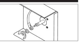
Connect the ring terminal wire lead to the probe terminal stud and secure with the lock washer and wing nut provided. *With the power removed*, proceed with installation and wiring according to Method A or B described on next page.
