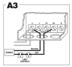
**Connect** terminal 2 to burner circuit neutral. Connect terminal P2 to burner circuit in series with other limit controls. Consult boiler manufacturer instructions for proper terminal connections. Control should be wired in series with and before other circuits.
