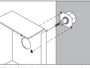
Slide keyhole slots over probe mounting screws and tighten screws (with either a 1/4" hex head driver or flat screwdriver.
