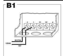
**Connect** the hot lead of the input voltage (120 VAC, 60 HZ) to terminal 1. Connect the neutral lead to terminal 2. 120 VAC, 60 HZ must be supplied to terminals 1 and 2 for internal operation of the control.
