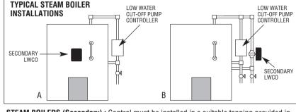
**STEAM BOILERS (Secondary)**: Control must be installed in a suitable tapping provided in the boiler(A), or in an equalizing line(B). The control should be located below the level of the primary low water cut-off but above the lowest permissable water line as specified by the boiler manufacturer.
