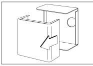
Loosen the two control box cover binding head screws and remove the cover.
