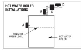
**HOT WATER BOILERS:** Probe must be installed at or above the minimum safe water level established by the boiler manufacturer. The probe may be installed directly in the boiler (A) if a suitable tapping is available, in the riser (B), in the header horizontally (C), or in the header vertically (D). **IMPORTANT:** To assure proper drainage, pipe diameter should be no less than 1" on installations in vertical piping and no less than 1½" on installations in horizontal piping.
