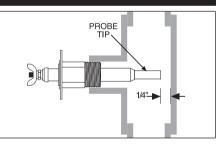
Check to insure 1/4" clearance from probe to *any* surface within the boiler or tee. When installed in a tee, the probe tip should extend fully into the pipe run. Apply pipe sealing compound to threads.
