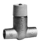
Sparco FlowChecks prevent the flow of water to any part of a system when the pump is shut off. They permit summer/winter operation of indirect water heaters. Sparco Flowchecks are easy to clean. Just unscrew the top of the valve for inspection and cleaning. Bronze and brass construction. To allow gravity flow, the Flowcheck can be changed to manual operation by turning the hand wheel counterclockwise (open position).
