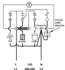
Wiring using 120V or 240V single phase line with auxiliary fan circuit.
