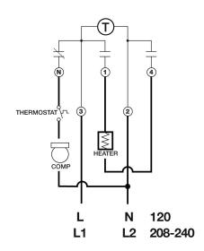
Fan and compressor loads not to exceed 2 hp. Heater not to exceed 4000 watts at 120V AC or 8000 watts at 240V AC.
