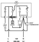
Wiring using differential of SPDT thermostat to delay fan after defrosting.
