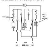
Wiring using 240V single phase line breaking both sides of heater circuit.
