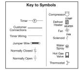
Wiring using 120V or 240V single phase line hot gas solenoid valve voltage common to timer. Refrigeration Cycle: Fan ON, hot gas solenoid valve closed, compressor ON. Defrost Cycle: Fan OFF, hot gas solenoid valve open, compressor ON.
