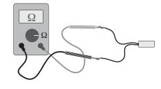
Do not apply voltage to a sensor at any time as damage to the sensor may result.
