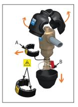
To purge the ferrous impurities in the steel DIRTMAG, the flexible magnetic stack is removed from the brass dry-well and, with the system still running, the drain valve is opened. Aided by the system pressure, the dirt and ferrous impurities, including magnetite flushes out quickly and effectively.
