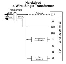
\* Common wire connection optional with batteries installed.
