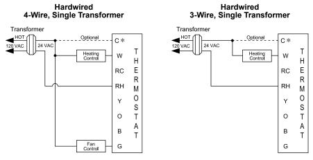
\* Common wire connection optional with batteries installed.
