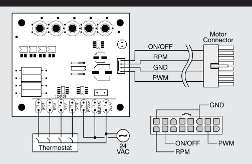
\*\* Note: For Hoffman 764-ECM 4-speed controller, the following connector changes are required: 3-640441-4 (output) and 1/4" quick connect (inputs).
