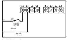
STEP 1 Connect 120 VAC Hot to terminal L1. Connect 120 VAC Neutral to terminal L2. Disconnect means and overload protection as required (provided by others).
