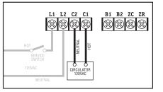
**STEP 2** Connect the circulator to C1 and C2. (C2 is neutral.)
