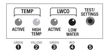
**1** TEMP **ACTIVE** Indicates that the HydroStat control is powered and that the temperature function is active.
