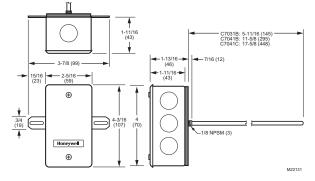
Fig. 1. C7041B,C Dimensions in in. (mm).
