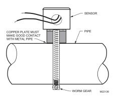
Fig. 6. Strap-on Mounting of Sensor.
