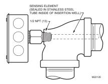
Fig. 3. Method of Mounting C7031D/C7041D Sensor.
