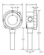
Fig. 2. C7021F, C7031G, C7041F, T775-SENS-OAT Dimensions in in. (mm).
