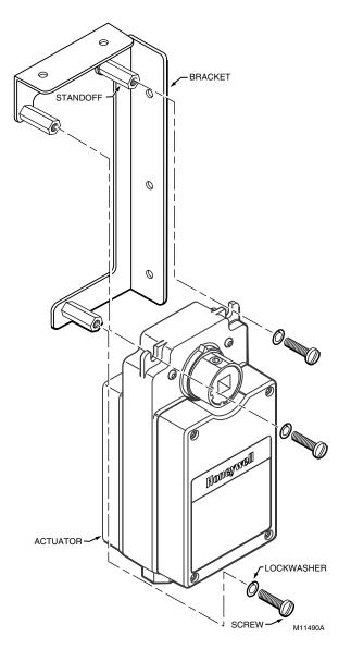
Fig. 2. Mounting the DCA on bracket using standoffs.
