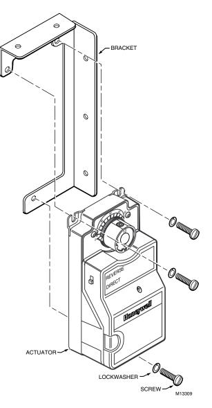
Fig. 3. Mounting a high torque DCA on bracket.
