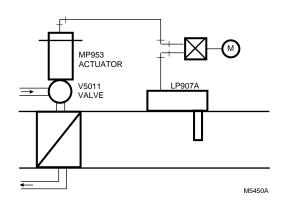
Fig. 4. Typical operation of duct mounted LP907.
