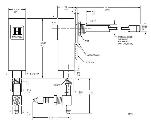
Fig. 1. Dimensions of LP907A in inches (millimeters).
