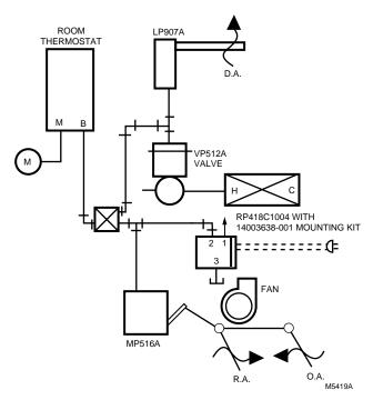
Fig. 2. Typical operation.
