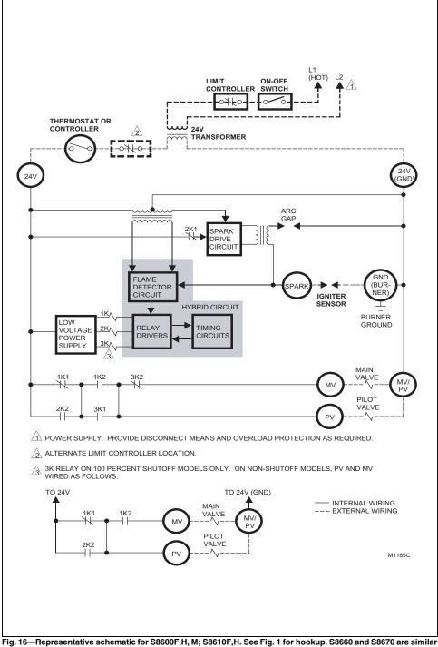
except the timing circuit includes a purge timer. See Fig. 6 for hookup.
