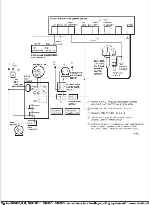
Fig. 8—S8600F,H,M; S8610F,H; S8660D; S8670D connections in a heating-cooling system with power-assisted combustion.
