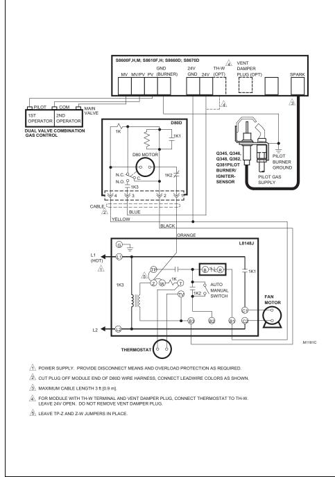
Fig. 9—S8600F,H,M; S8610F, H; S8660D; S8670D connections in a hydronic heating sytem with a D80D vent damper.
