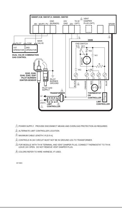
Fig. 7—S8600F,H,M; S8610F,H; S8660D; S8670D in a heating system with an atmospheric burner and a D80B vent damper.
