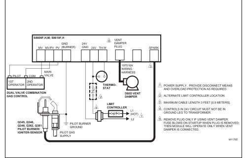
Fig. 2—S8600F,H,M; S8610F,H with a vent damper plug in a heating system with an atmospheric burner and a D80D vent damper.
