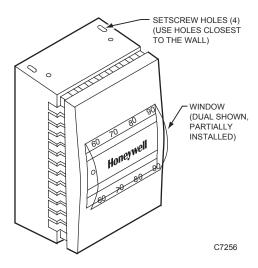
Fig. 2. Installation of window insert
