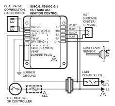
POWER SUPPLY. PROVIDE DISCONNECT MEANS AND OVERLOAD PROTECTION AS REQUIRED. MAKE SURE L1 AND L2 ARE NOT REVERSED; THIS WOULD PREVENT FLAME DETECTION.
