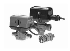
These 2-position (open/close) control actuators are used with VCZ1000, 1100, 6000 and 6100 series hydronic valves in a normal indoor environment to provide quick opening/closing to control the flow of hot and/or chilled water or glycol solution to 60% concentration. They are designed for on-off "zone" control of heating/cooling systems, or to control individual fan coil, baseboard radiator or convector applications.
