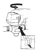
Fig. 2. Latch mechanism to detach actuator.
