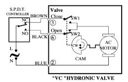
Fig. 8. Actuator wiring for SPDT Controller (Series 20 and 60).
