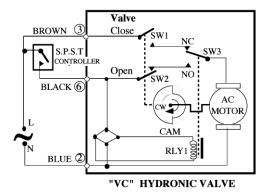
Fig. 9. Actuator wiring for SPST Controller (Series 40 and 80).
