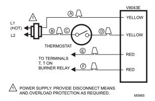
Fig. 30. Wiring a V8043F to a Flair System. (Wires are identified with letters to correspond with wires on Fig. 29.)
