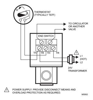
Fig. 15. Typical wiring for V8043F.
