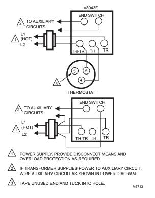
Fig. 34. Wiring a V8043F to a White-Rodgers System (1 option).
