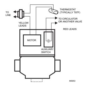
Fig. 14. Typical wiring for V8043E, V8044E.
