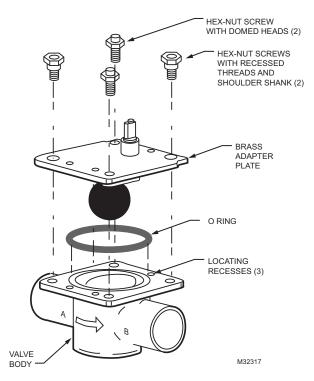
Fig. 11a. Install 40003918 conversion kit with brass adapter plate.
