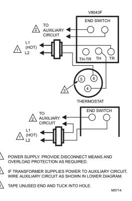
Fig. 35. Wiring a V8043F to a White-Rodgers System (alternate option).
