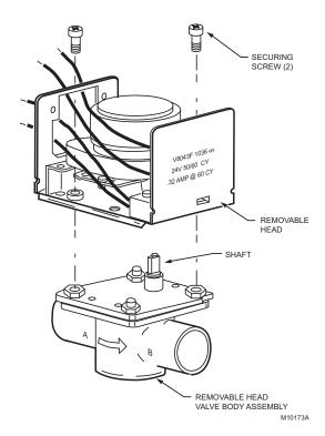
Fig. 12. Install new powerhead.
