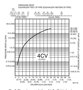
Fig. 6. Flow characteristics of 4 Cv (3.4 kv) valve.
