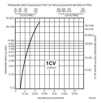
Fig. 3. Flow characteristics of 1 Cv (0.86 kv) flow.
