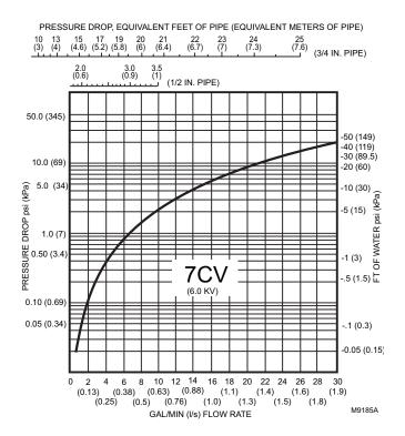
Fig. 7. Flow characteristics of 7 Cv (6.0 kv) valve.
