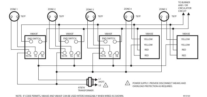
Fig. 22. Typical 5-zone system. Use an AT87A transformer to power up to 5 more zone valves.
