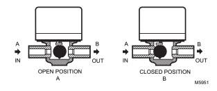
Fig. 36. V8043 operation for normally closed valve.
