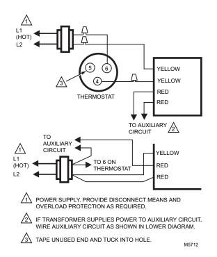
Fig. 33. Wiring a V8043E to a White-Rodgers System.
