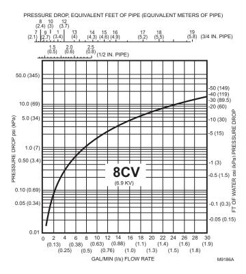
Fig. 8. Flow characteristics of 8 Cv (6.9 kv) valve.
