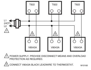
Fig. 16. T822 thermostat, V8043A valve hookup.
