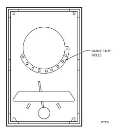
Fig. 5. Range stop installation.
