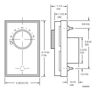
Fig. 1. Nominal dimensions in in. (mm).
