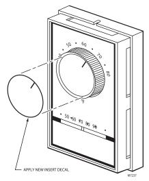
Fig. 6. Thermostat recalibration.
