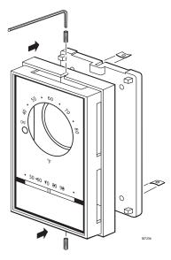
Fig. 4. Locking cover installation.
