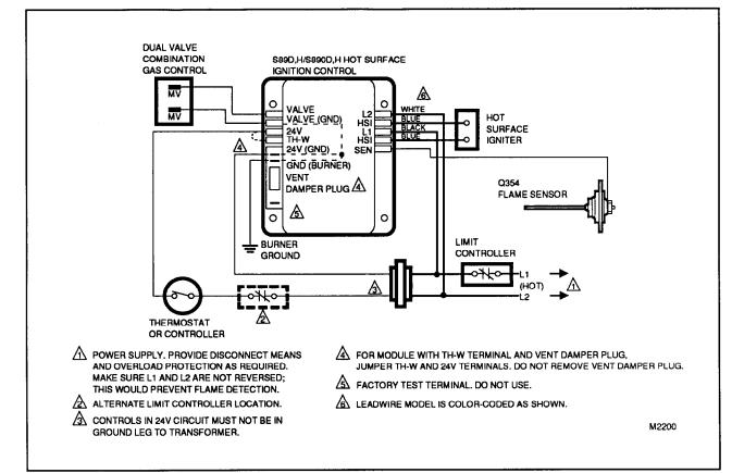
FIG. 3-S89D,H AND S890D,H IN AN ATMOSPHERIC BURNER HEATING SYSTEM.
