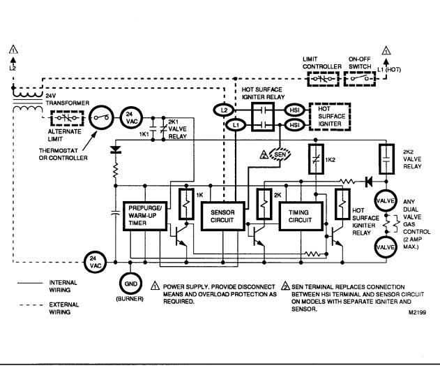
FIG. 14-S89/S890 SIMPLIFIED SCHEMATIC.
