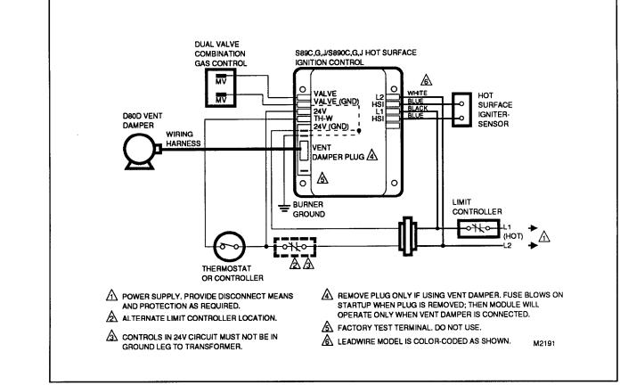
FIG. 4—S89C, G, J AND S890C, G, J IN AN ATMOSPHERIC BURNER HEATING SYSTEM WITH THE D80D VENT DAMPER.
