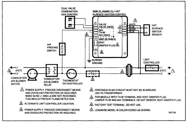
FIG. 6-S89C,G,J AND S890C,G,J IN A FAN-ASSISTED COMBUSTION HEATING SYSTEM.
