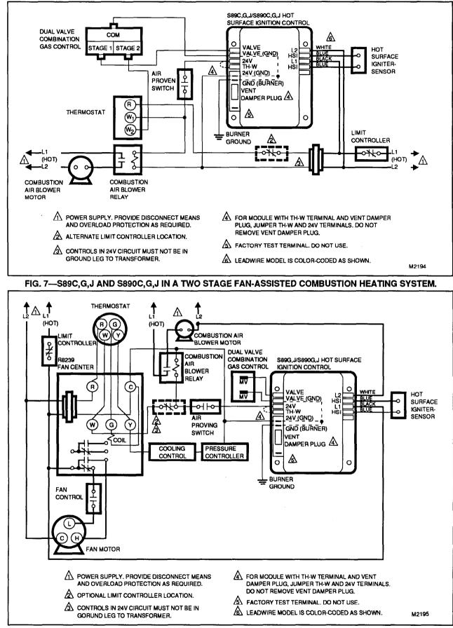
FIG. 8—S89C,G,H AND S890C,G,H IN A FAN-ASSISTED COMBUSTION HEATING-CENTRAL COOLING SYSTEM.
