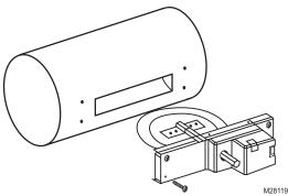
Fig. 9. Installing retrofit round damper.
