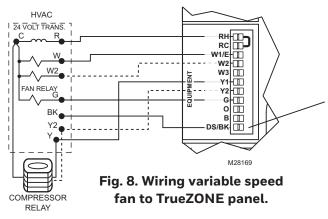
If using a Resideo TrueZONE panel, the panel's DS/ BK terminal is intended for use with a variable-speed fan. When one zone is calling (or less than 25% of capacity on systems with more than 4 zones), this terminal will be de-energized of 24 VAC. This reduces blower speed on most variable speed blowers.
