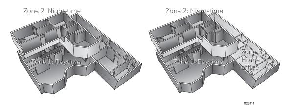
Fig. 3. Typical residential layout with multiple zones on one HVAC system.
