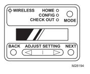
After checkout mode you should make a call for heat or cool from each thermostat to verify correct communication to the zone panel. Also, verify CPRD relief damper is adjusted correctly (see "Setting the Regulator" on page 7).
