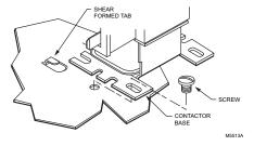
Fig. 1. Typical contactor mounting.
