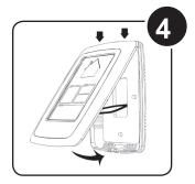
Attach front module to mounted back plate, first by hooking the top of the front module to the top clips of the back plate, then by pressing the bottom of the front module until you hear a 'click'.
