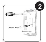
Guide the signal wires (2) through the central opening of the back plate and mount this plate to either a standard electrical device box or directly to the wall using screws. If required, use wall anchors.
