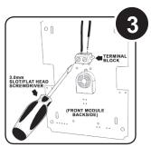
Insert signal wires (2) into the terminal block, located on the backside of the front module. Secure them in place by tightening the terminal screws using a small 3.0 mm slot/flat head screwdriver (not included).
