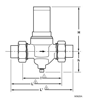
Fig. 1. DS05 installation dimensions in in. (mm).
