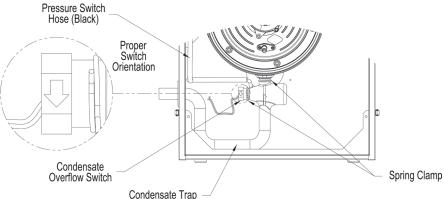
Figure 47: Condensate Overflow Switch Orientation
