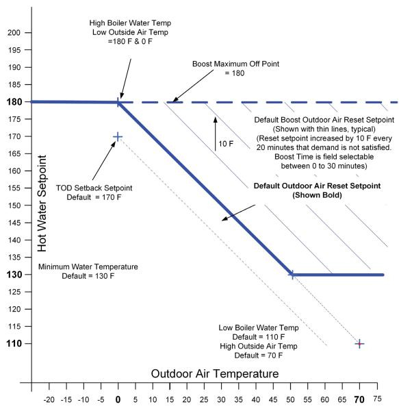
Figure 45: Outdoor Reset Curve - Typical for Central Heat and Auxiliary Heat
