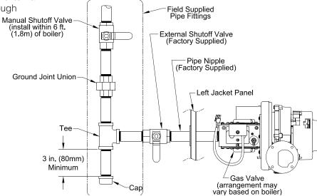
Figure 26: Recommended Gas Piping
