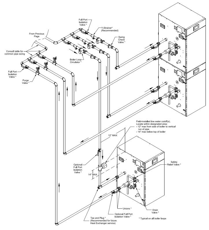
**NOTICE** Installing a low water cutoff in the system piping of multiple boilers is strongly recommended and may be required by Local Codes.
