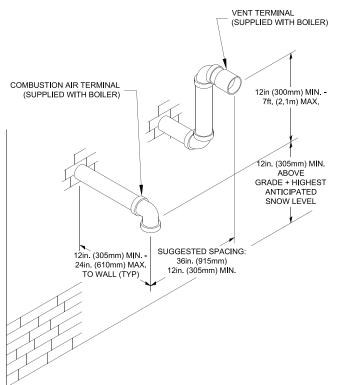
Figure 6A: Direct Vent - Staggered Vent and Air Intake Horizontal Sidewall Terminations
