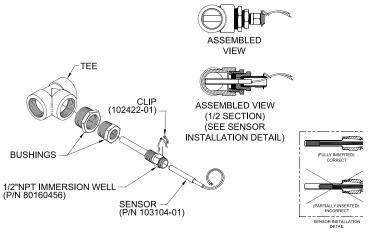
Figure 32: Recommended "Immersion" Type Header Sensor Installation Detail
