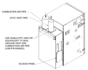
Figure 10B: Field Installation of CPVC Vent Pipe - Wall Mounted Boiler Builds
