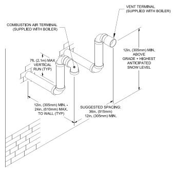
Figure 6B: Direct Vent - Snorkel Vent and Air Intake Horizontal Sidewall Terminations
