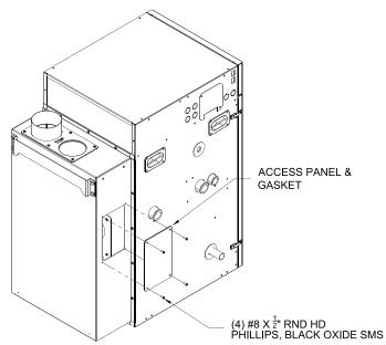
Figure 2E: Access Panel and Gasket Installation
