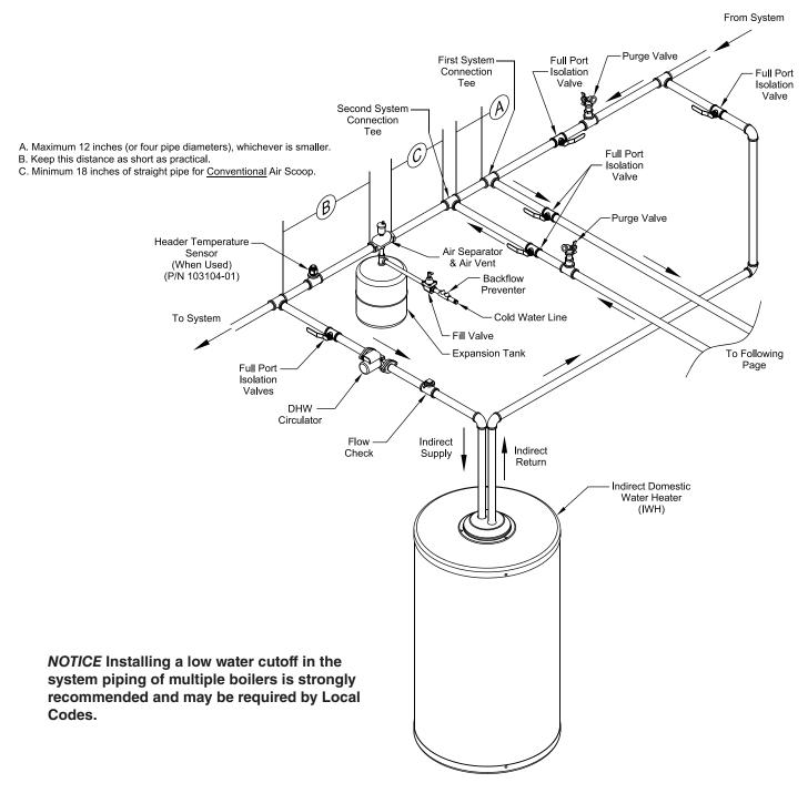
Figure 24A: Multiple Boiler Water Piping w/Domestic Hot Water Heater (Page 1 of 2)
