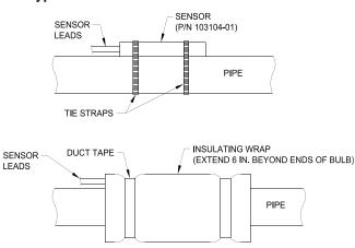
**Note:** The "Strap-On" type sensor must be mounted to the top side of a horizontal section of pipe as indicated in Figures 24A and 25A.
