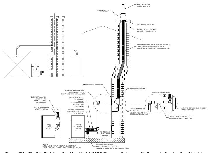
Figure 17A: Flexible Stainless Steel Vent in UNUSED Masonry Chimney with Separate Combustion Air Intake
