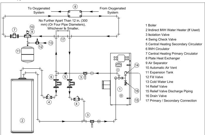
Figure 23: Isolation of the Boiler From Oxygenated Water with A Plate Heat Exchanger
