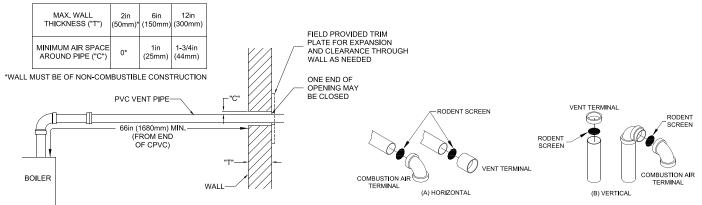
Figure 12: Wall Penetration Clearances for PVC Vent Pipe
