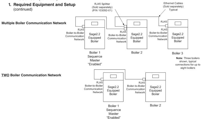
Figure 34: RJ45 Splitter Installation Detail
