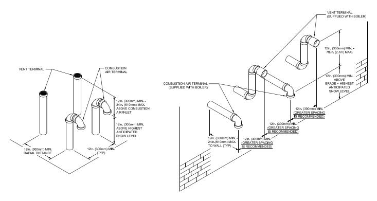
Figure 18: Multiple Boiler Direct Vent and Air Intake Terminations
