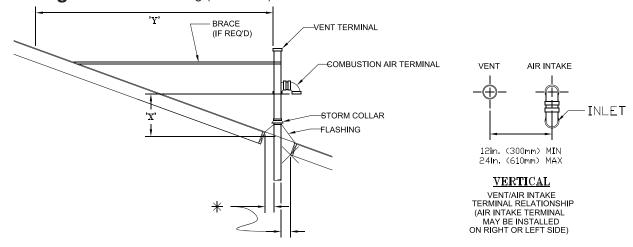
\* VENT PIPE MINIMUM CLEARANCE TO COMBUSTIBLE MATERIAL IS 1in. (25mm). COMBUSTION AIR PIPE MINIMUM CLEARANCE TO COMBUSTIBLE MATERIAL IS 7550
