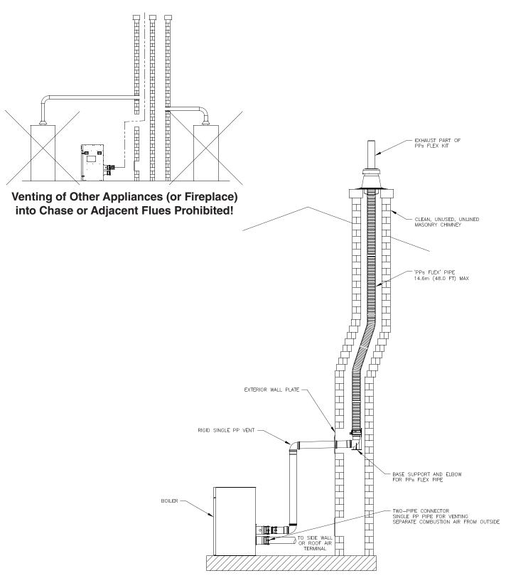
Figure 16A: Flexible PP Vent in UNUSED Masonry Chimney with Separate Combustion Air Intake
