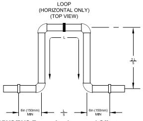
Figure 11: CPVC/PVC Expansion Loop and Offset
