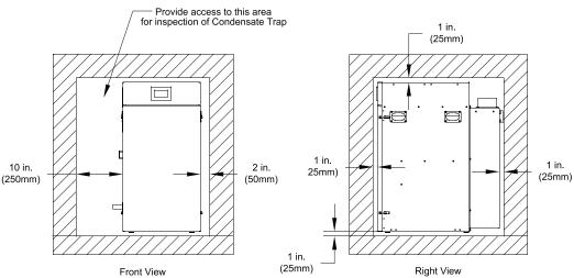
Figure 2B: Clearances To Combustible and Non-combustible Material, Wall Mounted
