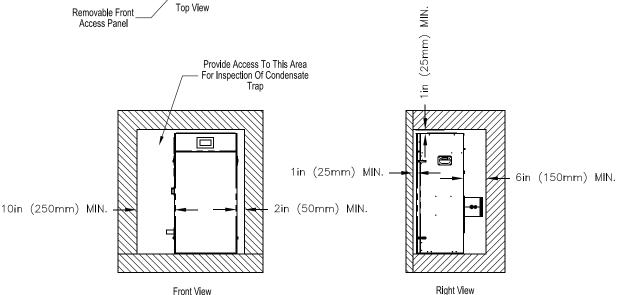
Figure 2A: Clearances To Combustible and Non-combustible Material, Floor Standing
