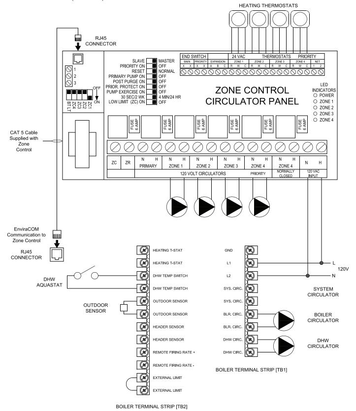
\*\*\*USE SAME POWER SOURCE FOR ALL CONTROLS AND ENSURE POLARITY TO ALL CONTROL DEVICES IS CORRECT
