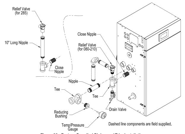
Figure 20: Factory Supplied Piping and Trim Installation
