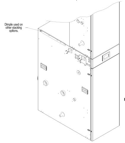
Figure 3: Stacking Boiler Attachment Bracket Placement
