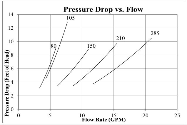
Table 13: Recommended Circulators for 50 ft. Equivalent ft. Near Boiler Piping [Approximately 20 ft. Straight Pipe, (4) 90° Elbows, and (2) Full Port Ball Valves]
