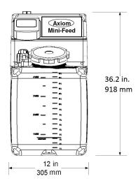
Depth – 12.0 in (305 mm) Clearances – Right/Left - 0 in (0mm) provided side screws on lid are removed upon installation Clearances – Top – 3" (75mm) Discharge ½" FNPT
