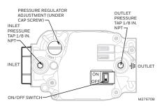
Fig. 3. Top view of VR8215S, T combination gas control.
