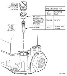
Fig. 5. Conversion kit installation in VR8205S, T and VR8215S, T series gas valves.
