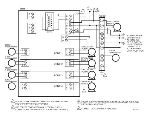
Fig. 7. R8888 Zone expansion using additional R8845U Universal Switching Relays.
