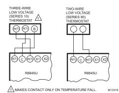
Fig. 8. R8845U thermostat connections.
