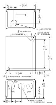
Fig. 1. R8845U dimensions in in. (mm).
