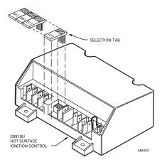
Fig. 2. Separating and installing selection tab.
