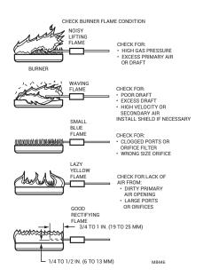
Fig. 6. Check burner flame condition.
