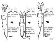
Fig. 2. Location of pilot burner.
