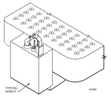
Fig. 5. Proper shielding of pilot flame.
