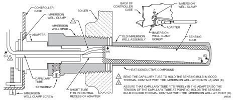
Fig. 3. Positioning the sensing bulb in the immersion well.
