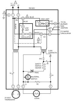
120 VAC POWER SUPPLY. PROVIDE DISCONNECT MEANS AND OVERLOAD PROTECTION AS REQUIRED.
