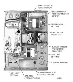
Fig. 4. Internal view of R8182D.
