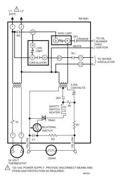
Fig. 8. R8182H internal schematic and wiring diagram.
