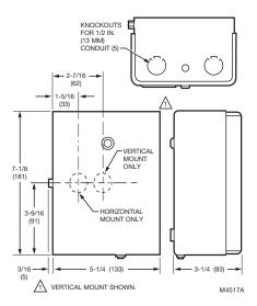
Fig. 1. R8182D installation dimensions in in. (mm).
