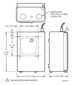
Fig. 2. R8182H installation dimensions in in. (mm).
