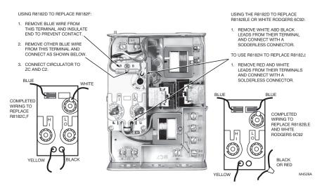
Fig. 6. Converting R8182D,H to replace other controls.
