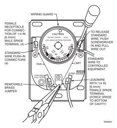
Fig. 5. Location of Wiring Connections.
