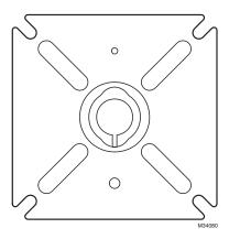
Fig. 3. Swivel mount (front view).
