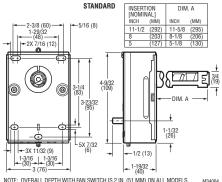
NOTE: OVERALL DEPTH WITH FAN SWITCH IS 2 IN. (51 MM) ON ALL MODELS.
