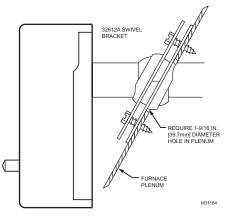
Fig. 2. Swivel mounting requires a 1-9/16 in. (40 mm) diameter mounting hole for element insertion.
