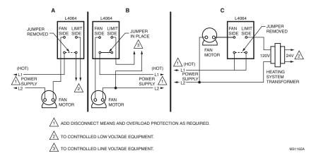
Fig. 4. Wiring Diagram for L4064.
