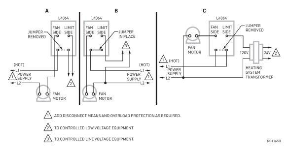
Fig. 11. A: LIMIT IN LOW VOLTAGE CIRCUIT.
