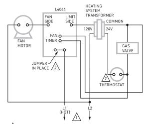
POWER SUPPLY. PROVIDE DISCONNECT MEANS AND OVERLOAD PROTECTION AS REQUIRED.
