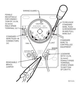
Fig. 9. LOCATION OF WIRING CONNECTIONS.
