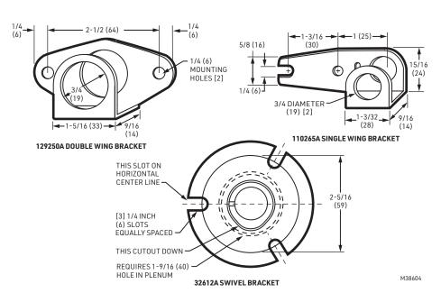
Fig. 2. MOUNTING DIMENSIONS IN in. [mm IN BRACKETS] OF BRACKETS.
