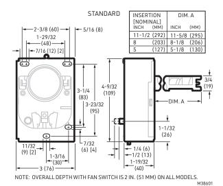
Fig. 1. MOUNTING DIMENSIONS IN in. [mm IN BRACKETS].
