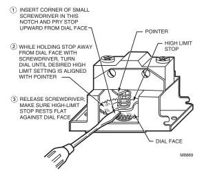
Fig. 15. Adjusting models with optional dial stop.
