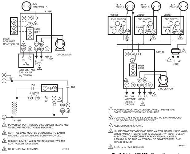
Fig. 7. External connections and internal schematic for L8148E.
