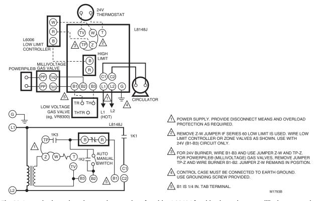
Fig. 13. Internal schematic and external connections for wiring L8148J for either low voltage or millivoltage gas valves.
