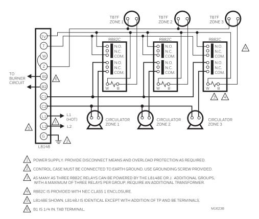
Fig. 14. Multizone system with R882C switched circulator.
