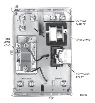
Fig. 2. Internal view of L8148A Aguasta® Relay.
