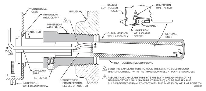
Fig. 4. Position of bulb in immersion well, and use of well adapter when required.
