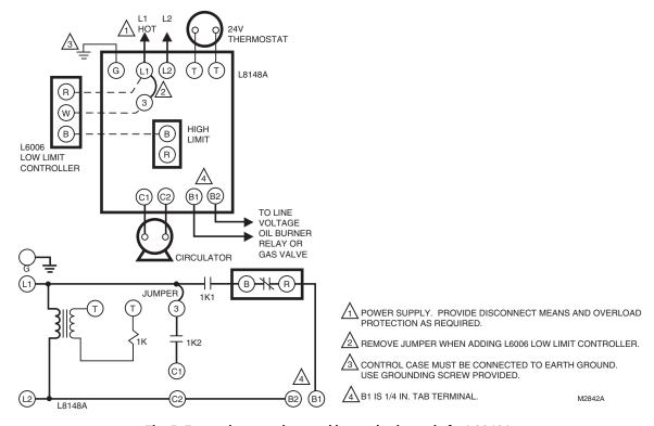
Fig. 5. External connections and internal schematic for L8148A.
