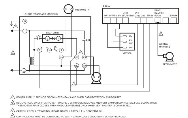
Fig. 11. Wiring L8148E with S8610A,F Intermittent Pilot Ignition Module with automatic vent damper plug and Resideo D892/M892 Vent Damper.
