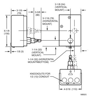
Fig. 1. L8148 dimensions in in. (mm).
