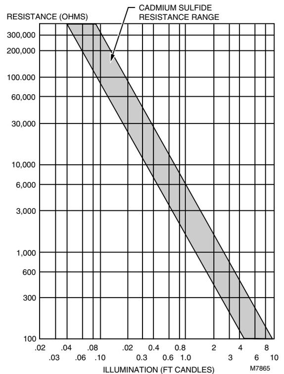
**Fig. 7. Light response tolerance for C554A cad cell.**
