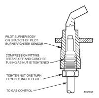
Fig. 3. Always use new compression fitting.
