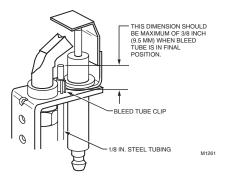
Fig. 4. Install bleed gas tube.
