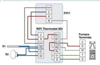
The WiFi Thermostat 562 operates a first stage radiant floor and a second stage fan coil for heating, and an air conditioner for cooling.
