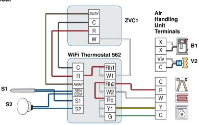
The WiFi Thermostat 562 operates a first stage baseboard/radiator and a second stage fan coil for heating, and an air conditioner for cooling.
