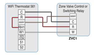
The WiFi Thermostat 561 operates a radiant floor heating system based upon the floor temperature sensor. The built-in air sensor is disabled.
