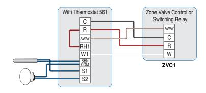
The WiFi Thermostat 561 operates a baseboard/radiator using an air temperature sensor. The air temperature sensor can be either built-in and/or external.
