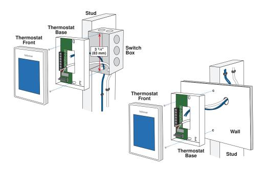
The WiFi Thermostat 561 operates a radiant floor heating system. The thermostat uses the built-in air temperature sensor.
