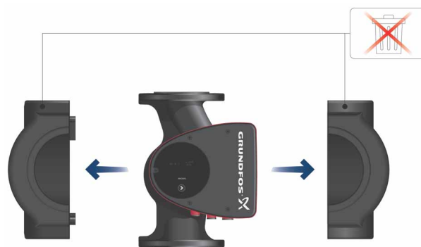
Fig. 3 Fitting insulating shells to the pump
