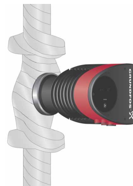
Fig. 12 Insulation of pump housing and pipework
