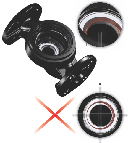
Fig. 11 Incorrectly centered sealing system
