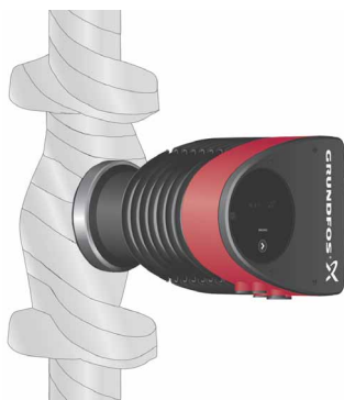
Fig. 13 Insulation of pump housing and pipework
