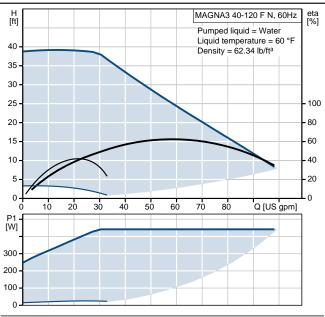
Maximum operating pressure: 174 psi Flange standard: GF GF15/26/40/43 Pipe connection: PN12 Pressure stage: Port-to-port length: 8 9/16 in Liquid: Pumped liquid: Water Liquid temperature range: 14 .. 230 °F 60 °F Liquid temp: Density: 62.34 lb/ft<sup>3</sup>
